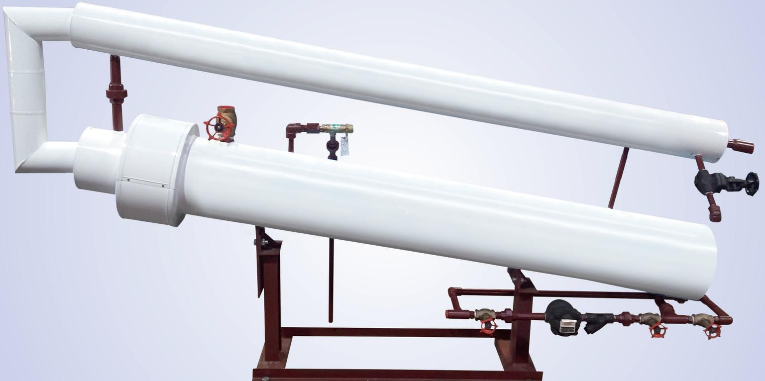
Steam heated vaporisers provide an easy and cost effective method of vaporising large quantities of liquid CO<sub>2</sub> to gas. Designed for direct connection to the outlet of a bulk storage tank, the steam vaporisers are available with nominal vaporisation capacities of 0.5 te/h, 1.0 te/h and 2.0 te/h.
